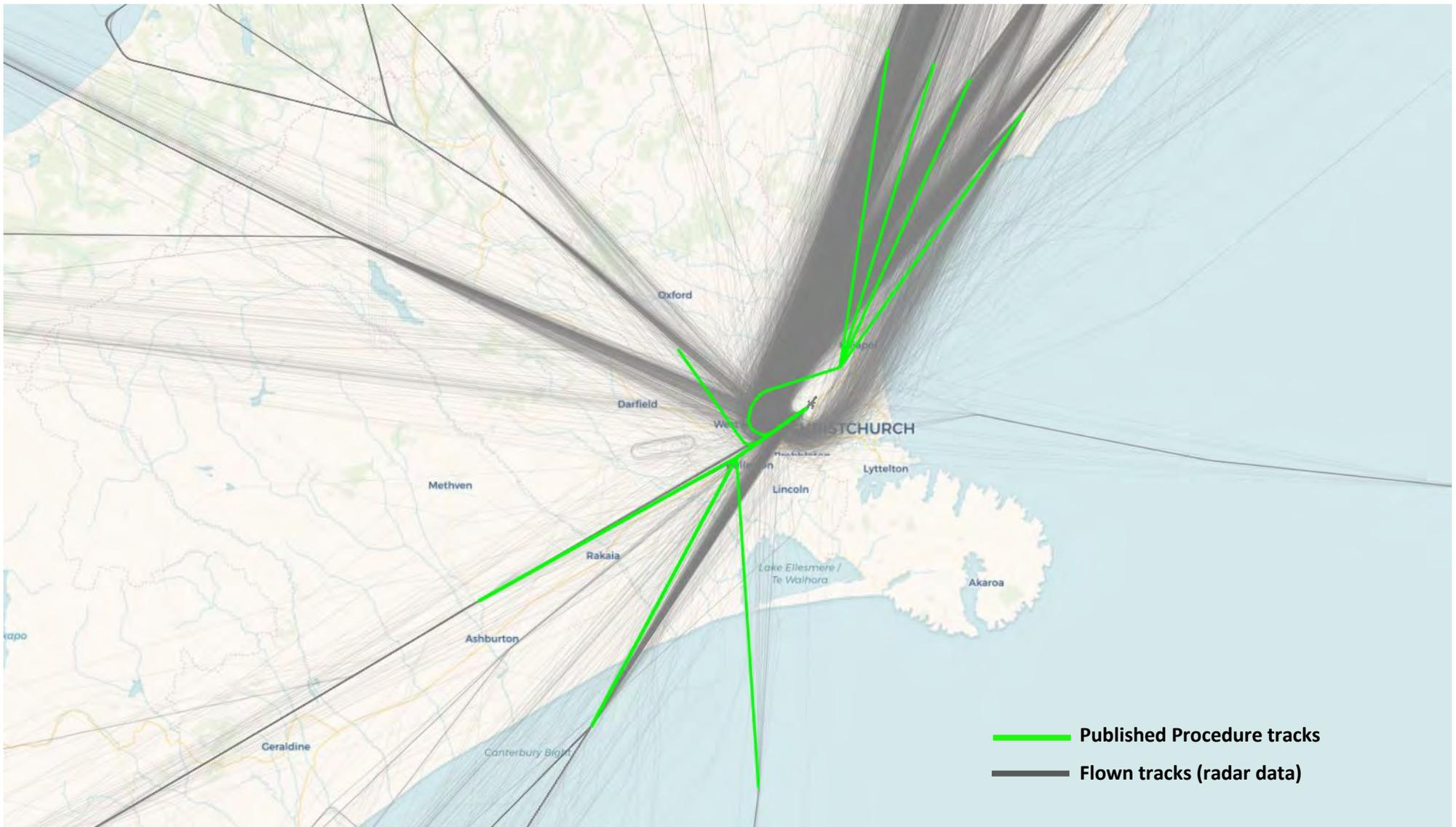
Figure 02-3 Runway 20 Departures Procedure vs Flown Tracks
