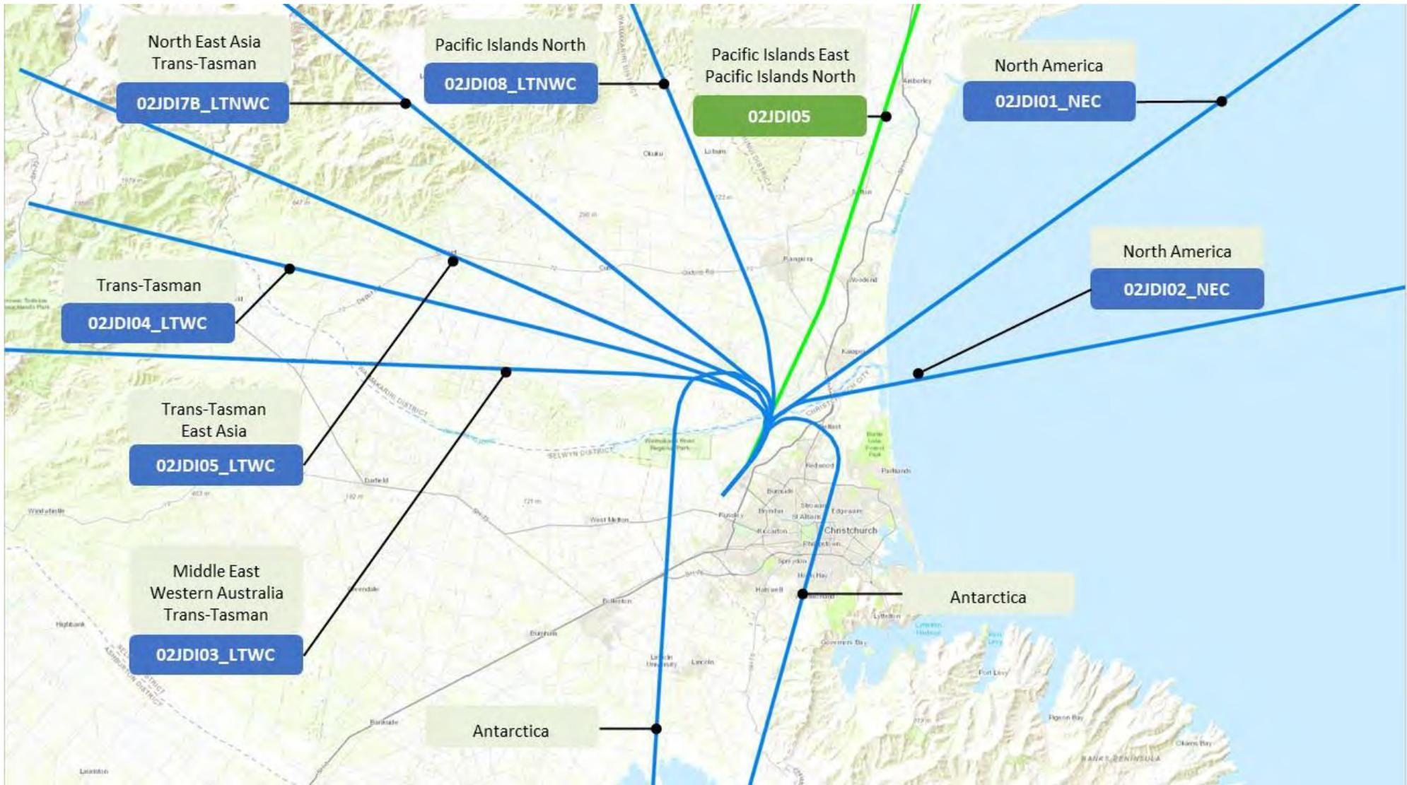
Figure 05-6 Runway 02 Jet International Departures Adopted Flight Tracks (Antarctica is not modelled)
