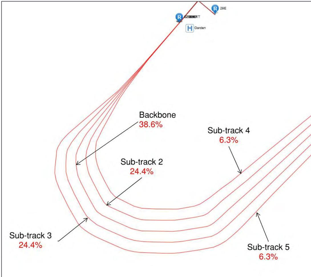
The distance between the backbone and each sub-track must be defined by the modeller at each point along the backbone track. There are standard settings in AEDT for allocating aircraft across dispersed tracks which concentrates more aircraft movements on the backbone and progressively fewer on the outer sub-tracks as shown in Figure 4. Table 2 lists the standard dispersion for 5 and 7 sub-tracks, these standard dispersion settings are based on a normal/Gaussian distribution.
