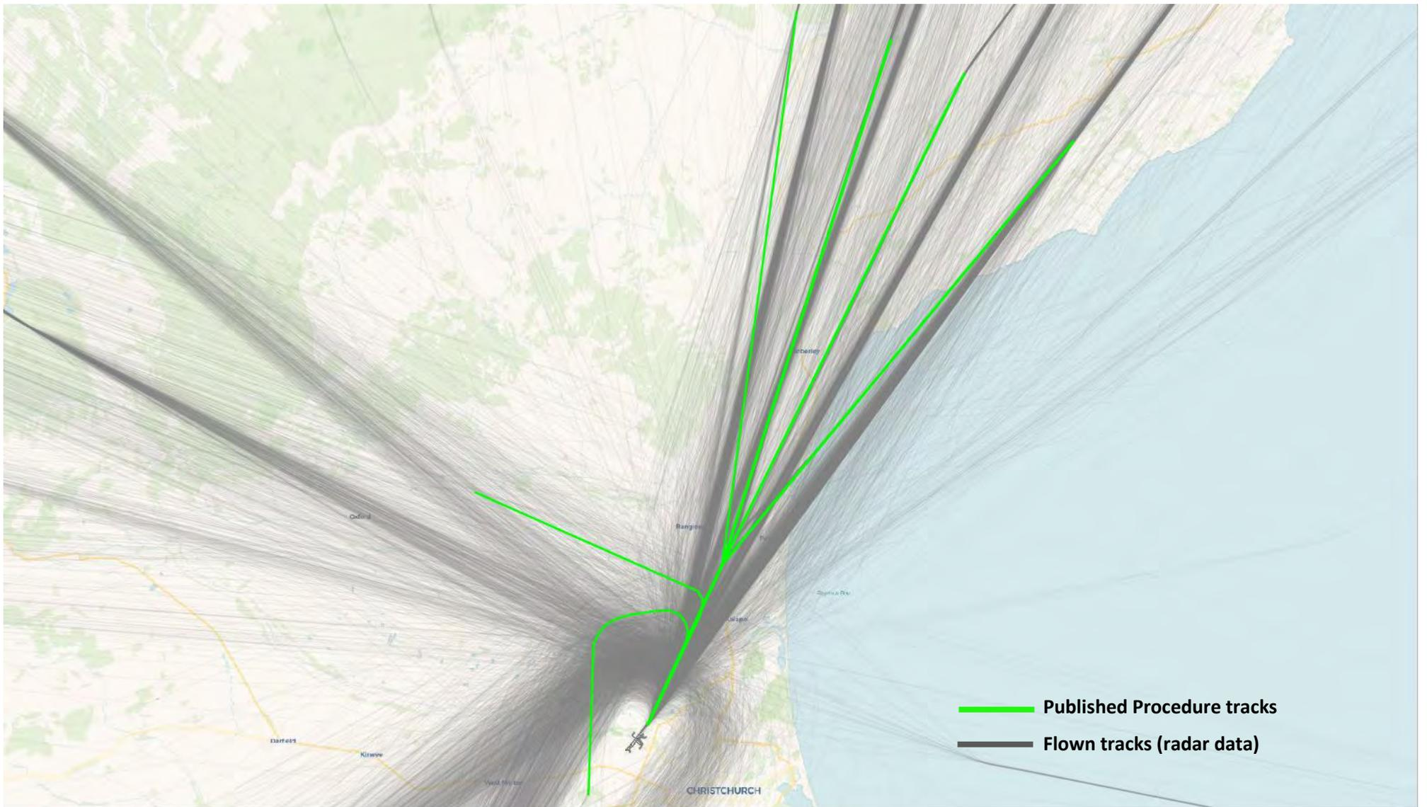
Figure 02-2 Runway 02 Departures Procedure vs Flown Tracks
