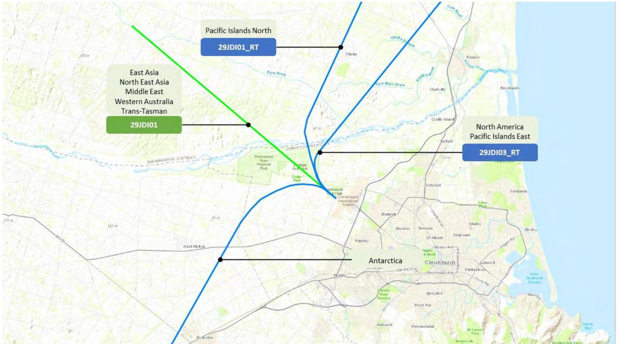
Figure 05-12 Runway 29 Jet International Departure Adopted Flight Tracks (Antarctica is not modelled)
