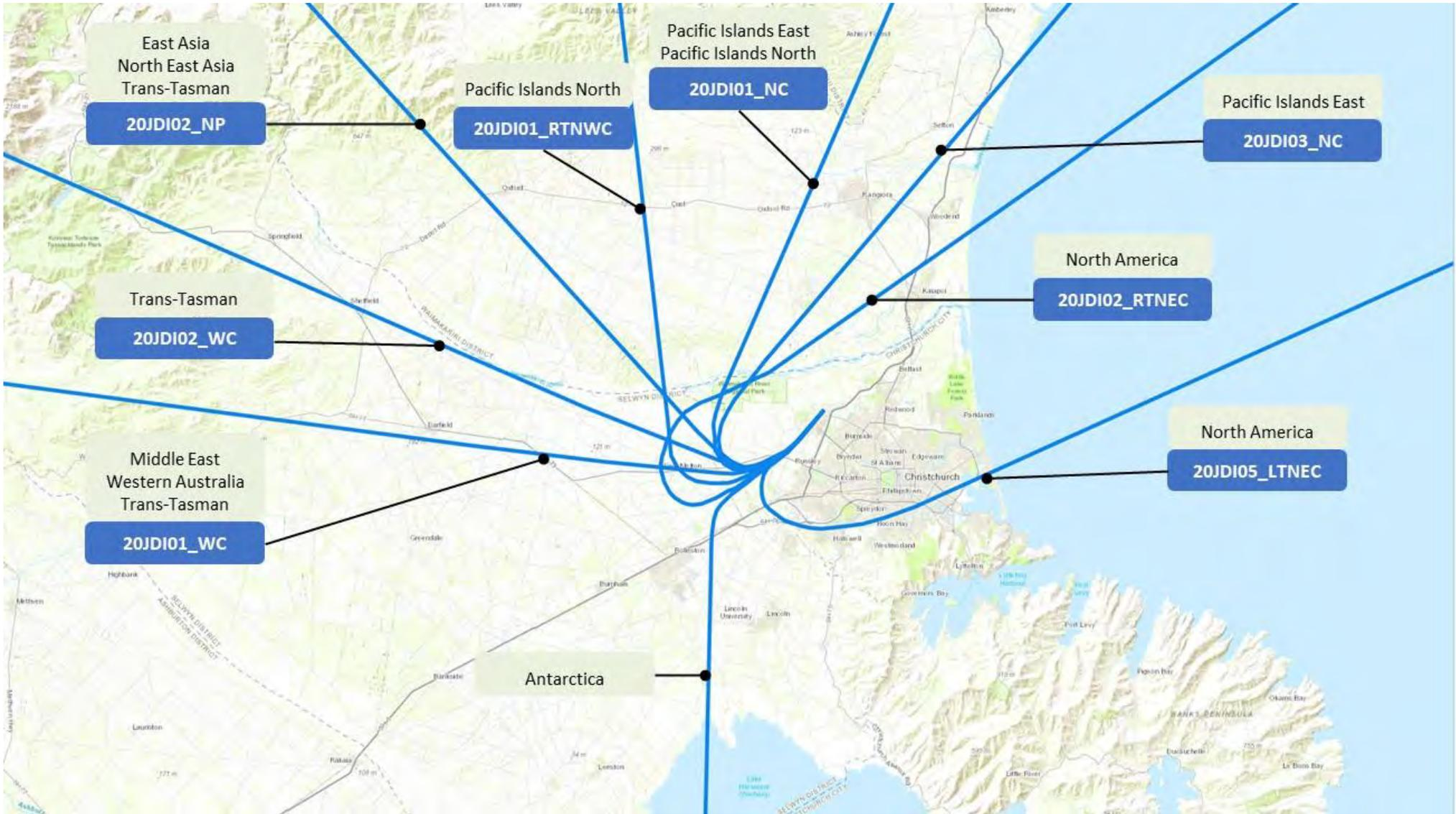
Figure 05-2 Runway 20 Jet International Departure Adopted Flight Tracks (Antarctica is not modelled)
