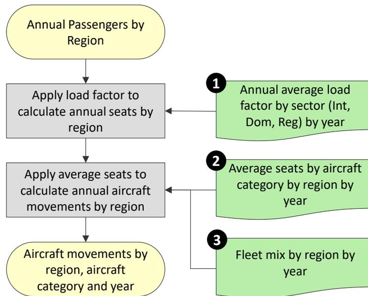
**Figure 06-1 Methodology to Calculate Annual Aircraft Movements**
