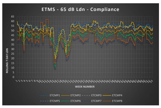
Graph 4.1: ETMS predicted 2020 noise levels for ETCMP 1 to ETCMP 8, located on the 65 dB  $L_{dn}$  engine testing contour
